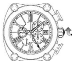
Turning the crown clockwise (upward): The hour hand is set back one hour.
