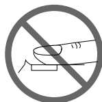
Finger too far back on the photosensor.
