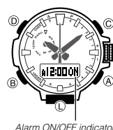
Alarm ON/OFF indicator
