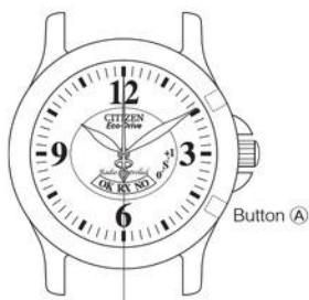
The second hand stops at the RX position.
