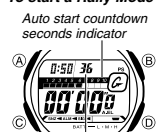
Remaining auto start countdown time (36 seconds indicated here)
