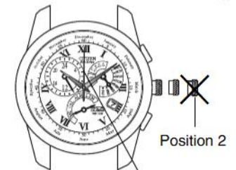
[Crown Pulled Out Too Far]
