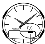
Power Saving indicator
