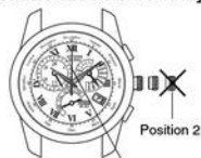
[Crown Pulled Out Too Far]
