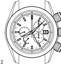
Example 2 Hour hand and calendar: Area B (New York) 24-hour hand: Area A (Japan)
