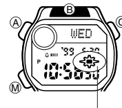
EL alarm on indicator
