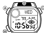
EL alarm on indicator
