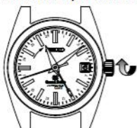
[Ex.1] Hour hand and calendar: Area A (Japan) 24-hour hand: Area B (New York)
