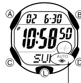
Auto light switch on indicator
