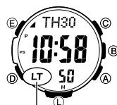
Auto light switch on indicator
