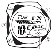
Auto light switch on indicator
