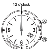
Correct hour and minute hand home position
