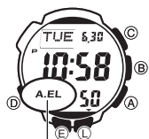
Auto light switch on indicator
