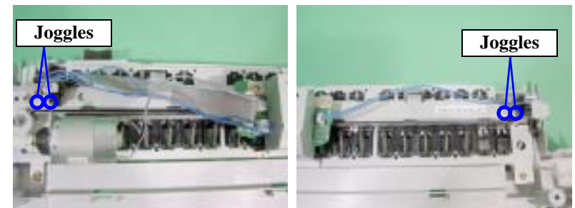
Figure 4-142. Reinstalling the Cutter Sensors
