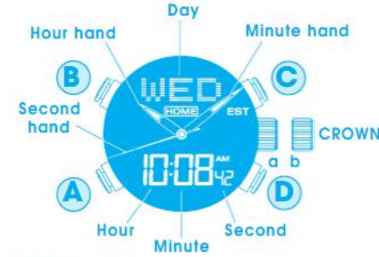
CROWN position a: normal position b: extended position (analogue time setting) (Caliber NX14)
