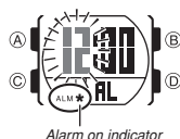
Alarm on indicator
