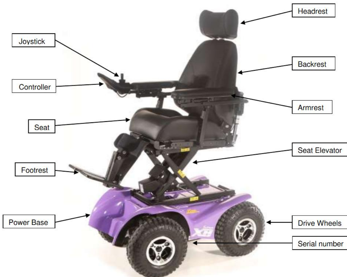
Figure 3 - Extreme X8 Major Components
