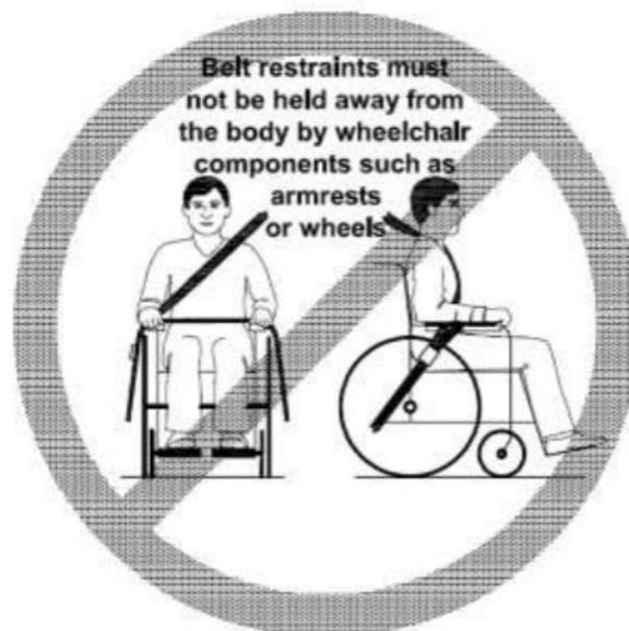
Figure 122 – Illustration of improper positioning of belt restraints
