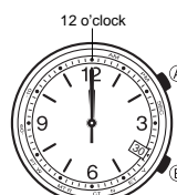
Correct hour and minute hand home position
