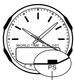
Power Saving indicator
